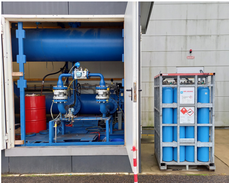
Figure 1. VSL's primary standard for the calibration of natural gas flowmeters on the left (see also Table 1), hydrogen cylinder bundle on the right. The primary standard was modified to the use of HENG in addition to natural gas.
